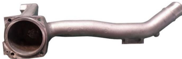
Gambar 1.1 Pipe Water Inlet EW010
