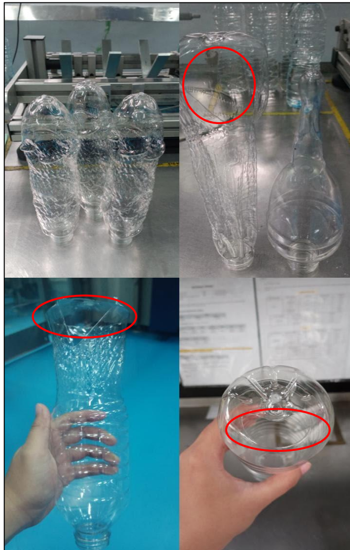
Gambar 1.1 Reject Preform Gagal Blow (Sumber : Data Pribadi)
