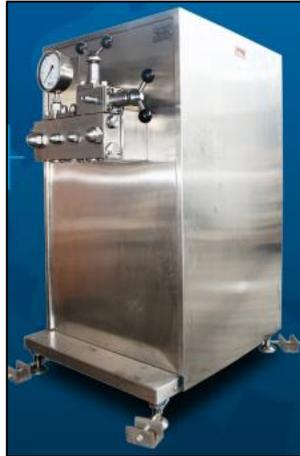
Gambar 2.10 Mesin *Homogenizer*
