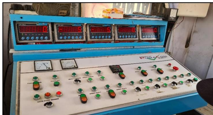
Gambar 2. 5 *Batching Plant Operator*
