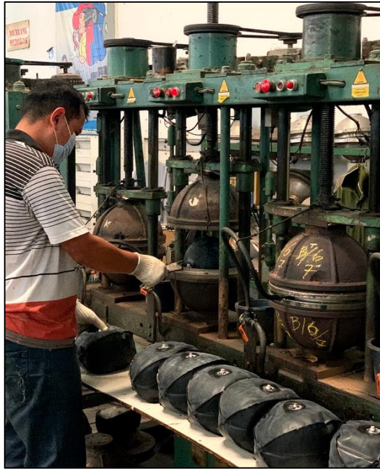
Gambar 4. 8 Vulkanisir Bola Bladder
