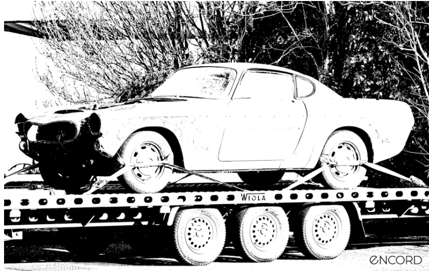
Gambar 2.5 Pengolahan citra Threshold pada kendaraan (sumber : https://encord.com/blog/image-thresholding-image-processing/ )
