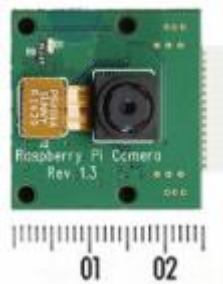
Gambar 2.5 Pi Camera v1 5MP (Sumber: Pomaska, 2019)
